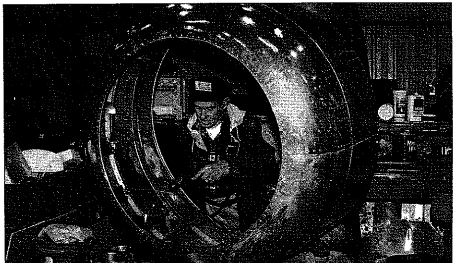
Ed Wochomurka, sheet metal expert, puts finishing touches on one of the restored engine nacelles.
